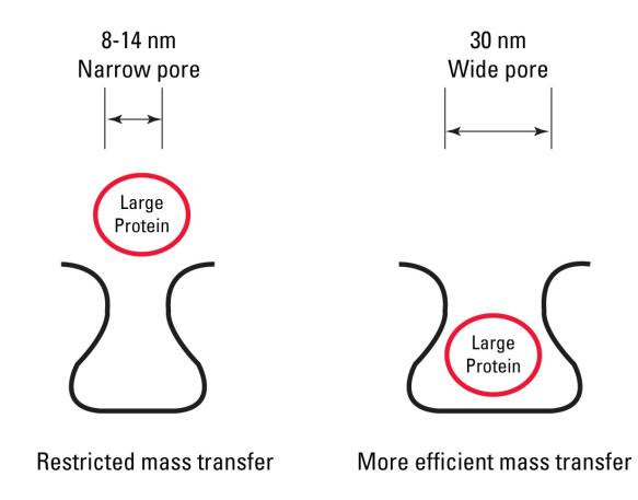
• The larger pore size of the TSKgel Protein C<sub>4</sub>-300 column helps in more efficient mass transfer during chromatographic analysis.
